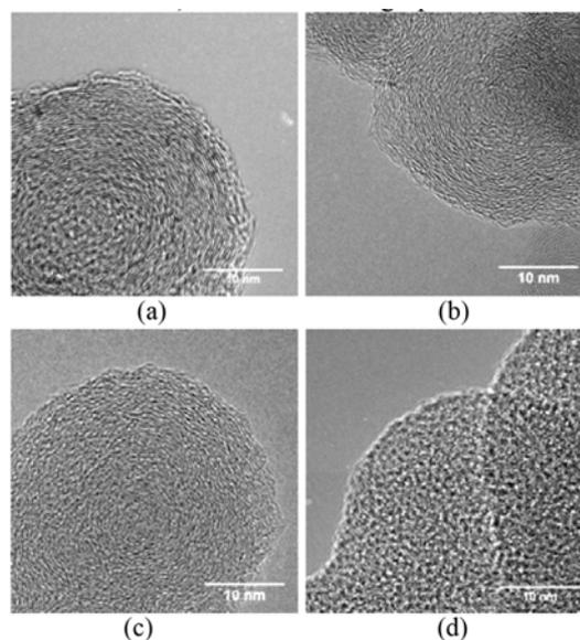
Figure 6. HRTEM images of various soot particles: (a) carbon black, (b) heavy-duty diesel engine, (c) light-duty DISI engine with gasoline, (d) light-duty DISI engine with E85 (Seong *et al.*, 2013) [Reprinted with permission from SAE paper 2013-01-2574 © 2013 SAE International].
