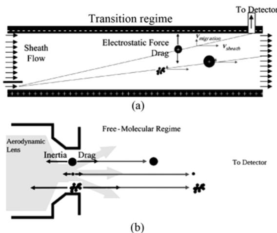
Figure 1. A schematic representation of the different diameter sizing measurements for: (a) DMA ( $d_m$ ) and (b) AMS ( $d_{wa}$ ). (DeCarlo *et al.*, 2004) [Reprinted from *Aerosol Sci. Technol.*, 38(12): 1185-1205, 2004, with permission from American Association for Aerosol Research (AAAR)].
