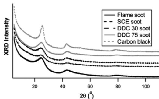
Figure 4. XRD patterns of various soot samples (SCE: single-cylinder diesel engine, DDC: multi-cylinder diesel engine) (Seong and Boehman, 2013) [Reprinted from *Energy Fuels*, 27(3): 1613-1624, 2013, with permission from American Chemical Society].
