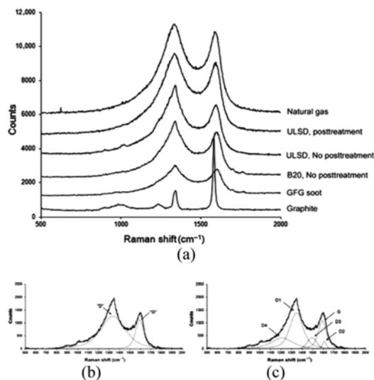
Figure 5. (a) First-order Raman spectra of various samples (vertically offset for clarity), (b) Typical curve fit for Raman spectra using two-band combinations, (c) Typical curve-fit for Raman spectra using five-band combinations (Soewono and Rogak, 2011) [Reprinted from *Aerosol Sci. Technol.*, 45(10): 1206-1216, 2011, with permission from American Association for Aerosol Research (AAAR)].
