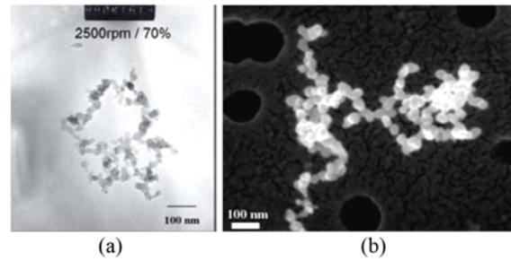
Figure 2. Diesel engine soot particle images taken by: (a) TEM (Lee *et al.*, 2003) and (b) SEM (Gwaze *et al.*, 2006) [Reprinted from *J. aerosol sci.*, 37(7): 820-838, 2006, with permission from Elsevier].
