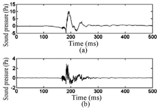
Figure 1. Door-slamming sound pressure signals of sample car No.1: (a) Original sound signal of door-slamming; (b) Sound signal of door-slamming extracted by the leaky integration.
