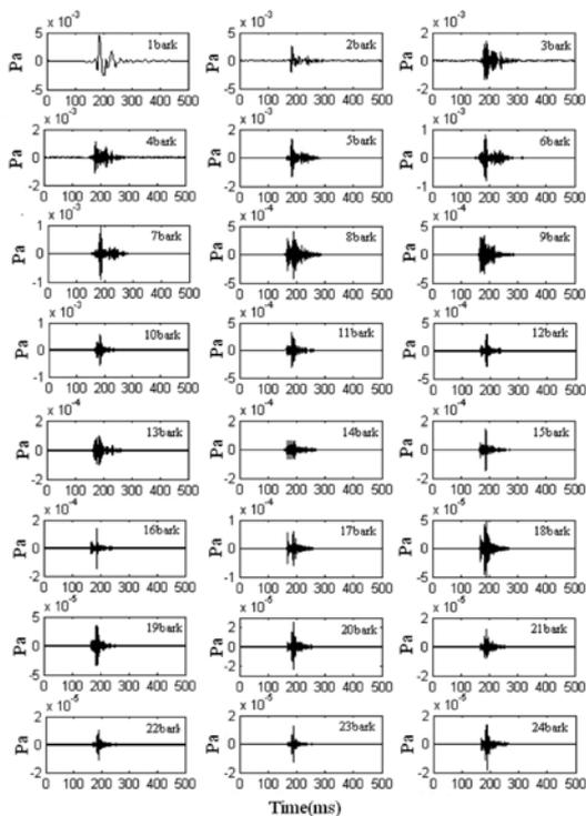
Figure 2. Decomposition results of the door-slamming sound pressure signal of sample car No.1 through critical-band-based wavelets.
