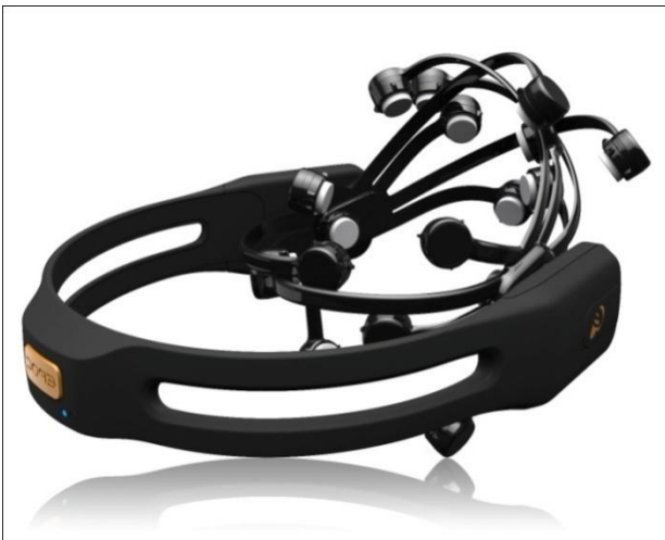
Fig. 4 Low-cost EEG signal acquisition hardware Emotiv EPOC Neuroheadset
