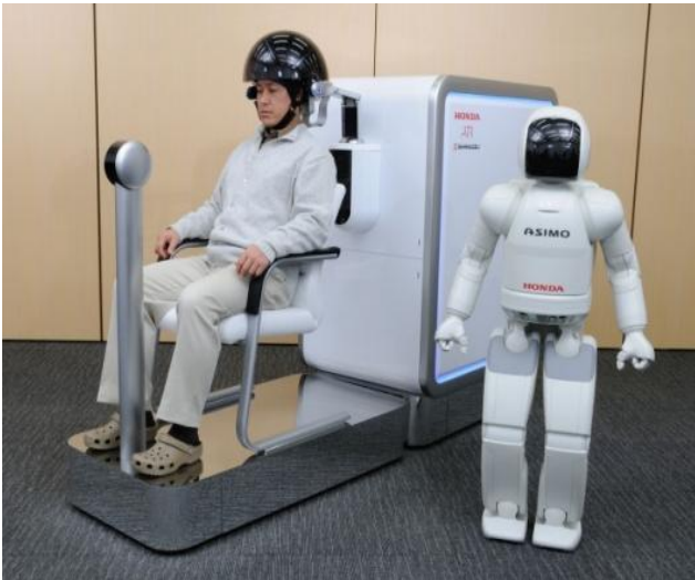
Fig. 1 Brain-Computer Interface used for control of humanoid robot Honda Asimo only with human thoughts. Source: Honda
