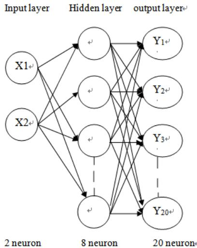
Fig.5. structure of neural network
