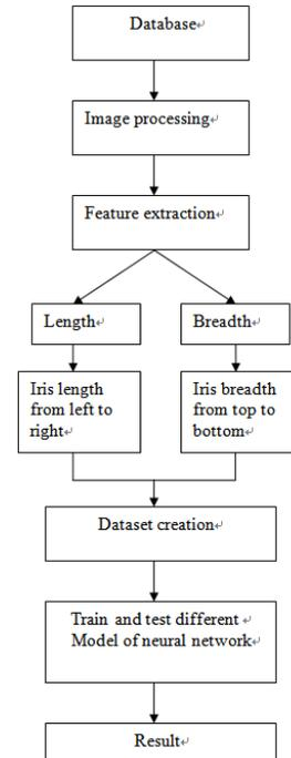
Fig.4.Flow graph of training and testing phase
