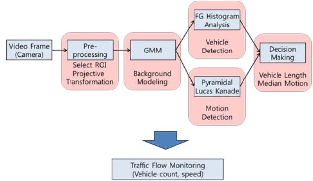
Fig. 2 Automatic vehicle detection and counting algorithm.
