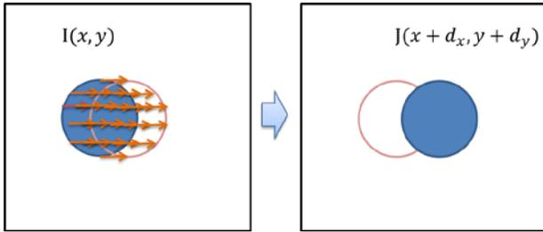
Fig.1 Illustration of optical flow.
